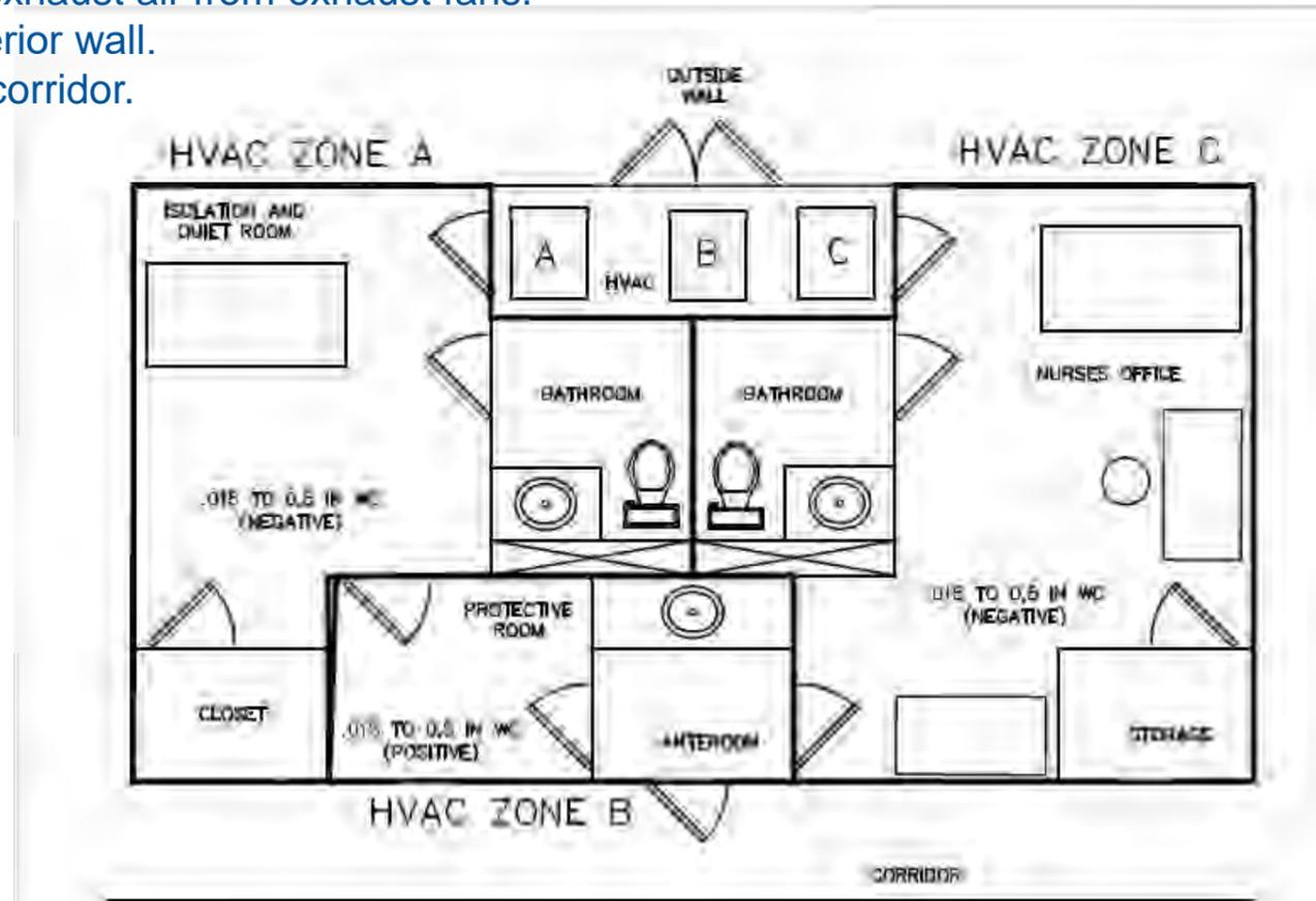
**Note:** Systems A, B, and C are the Dedicated "Isolation Mode" systems, each system is individually operated and controlled. The Supplementary HVAC systems for "Normal mode" are not shown.
