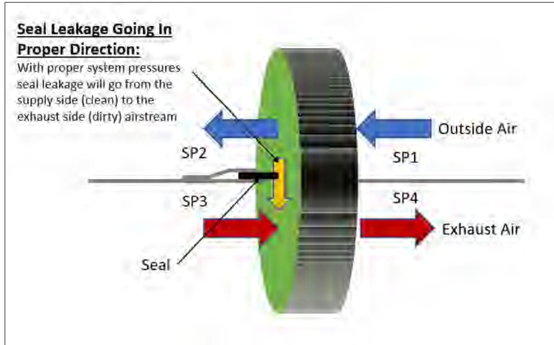
Figure 5 Supply static pressure should be higher than exhaust static pressure
